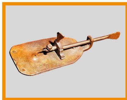
**Van Leeuwenhoek made** his microscopes himself. They comprised a tiny spherical lens held between two plates with a hole in each side and a pin to hold the specimen.
