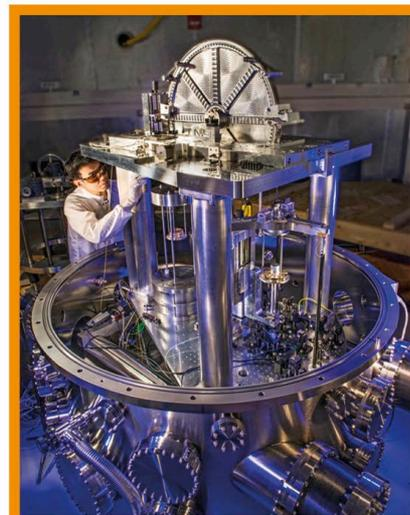
**The Kibble balance** at NIST produces incredibly accurate measurements, and has contributed to the recent redefinition of all base measurement units in terms of physical constants.
