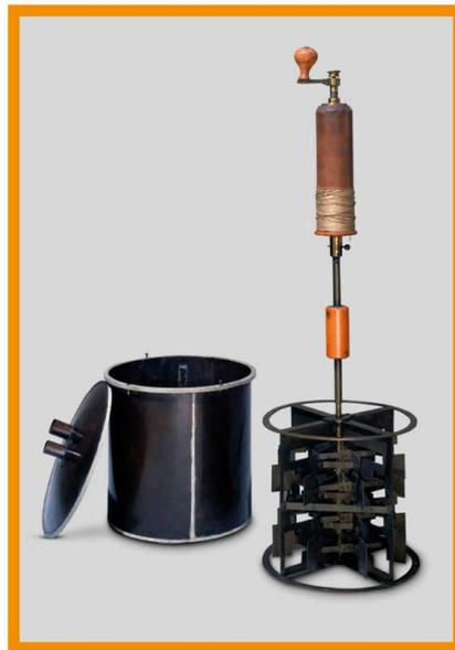
**For his experiment,** Joule used this vessel, filled with water, and the brass paddle wheel, turned by falling weights. The water’s rising temperature showed that mechanical work created heat.
